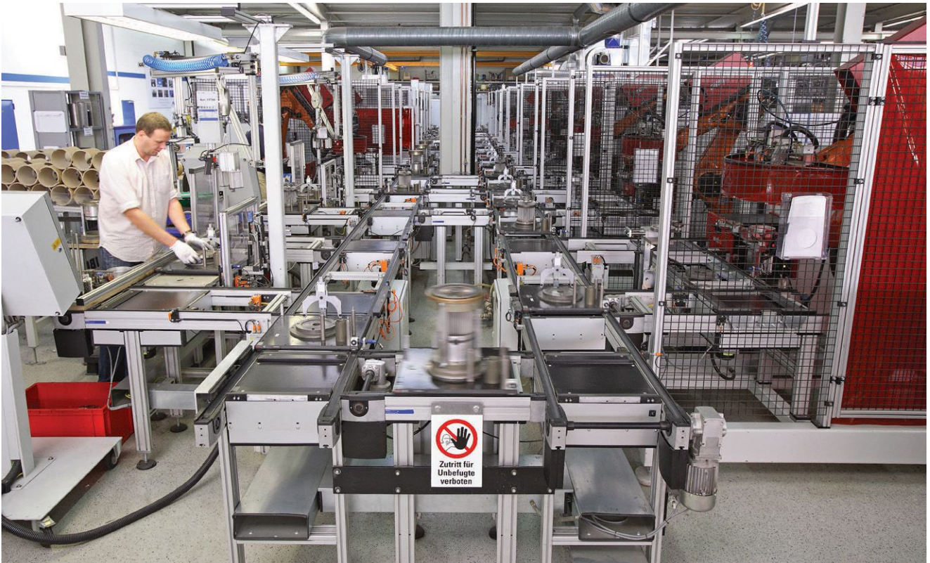
Conveyor-based automation moves parts through a guarded production line while an operator works at a manual station. (Provided by Bosch Rexroth)
