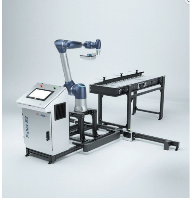
The new robotic palletizer Pallet EZ from Doig Corp., powered by OnRobot's D:PLOY platform, is an example of a complete, off-the-shelf robotic system. Unlike traditional automation systems that require weeks of integration and specialized expertise, Pallet EZ is ready to install and deploy the same day. (Provided by OnRobot)
