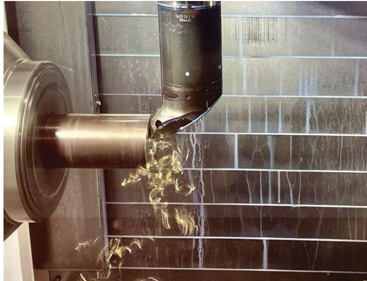
By outfitting an automated machining cell with modular Capto blocks and Sandvik Coromant Silent Tools, Acutec was able to prevent chip buildup around the cutting zone, eliminate chatter, stabilize processes and extend tool life. (Provided by Sandvik Coromant)
