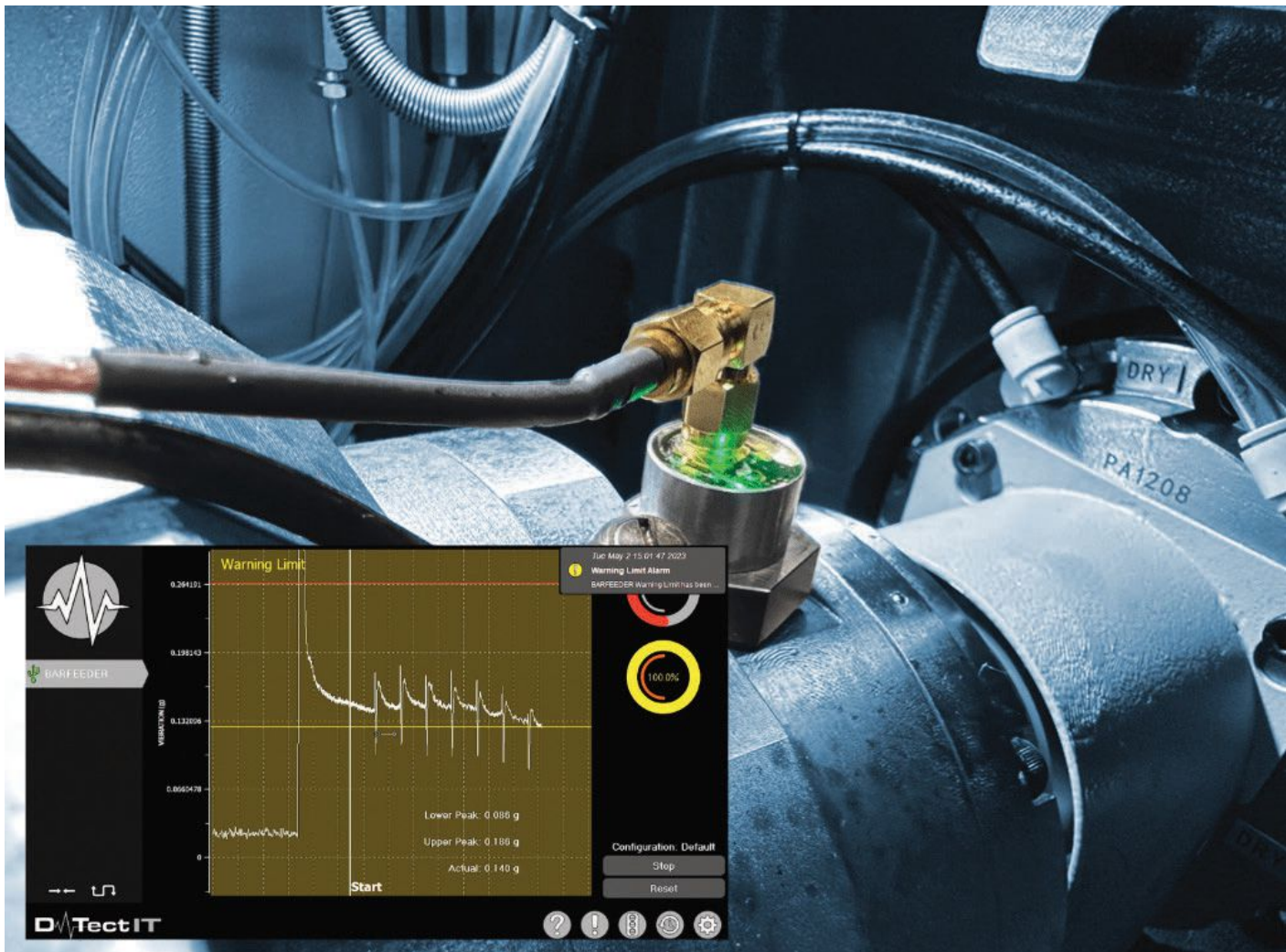
A vibration sensor is attached to the spindle used with Caron Engineering's DTest-IT to detect and control bar-feeder vibration automatically. (Provided by Caron Engineering)
